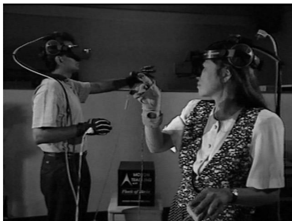
Figure 1 Two students interacting with a virtual ship via head-mounted displays and data gloves. Despite their physical proximity to one another, they are operating in completely different parts of the virtual ship.
