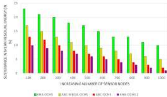
Figure 6. Proposed NIUS-HEHOA-OCHS: Sustenance in Mean Residual Energy under different network size
