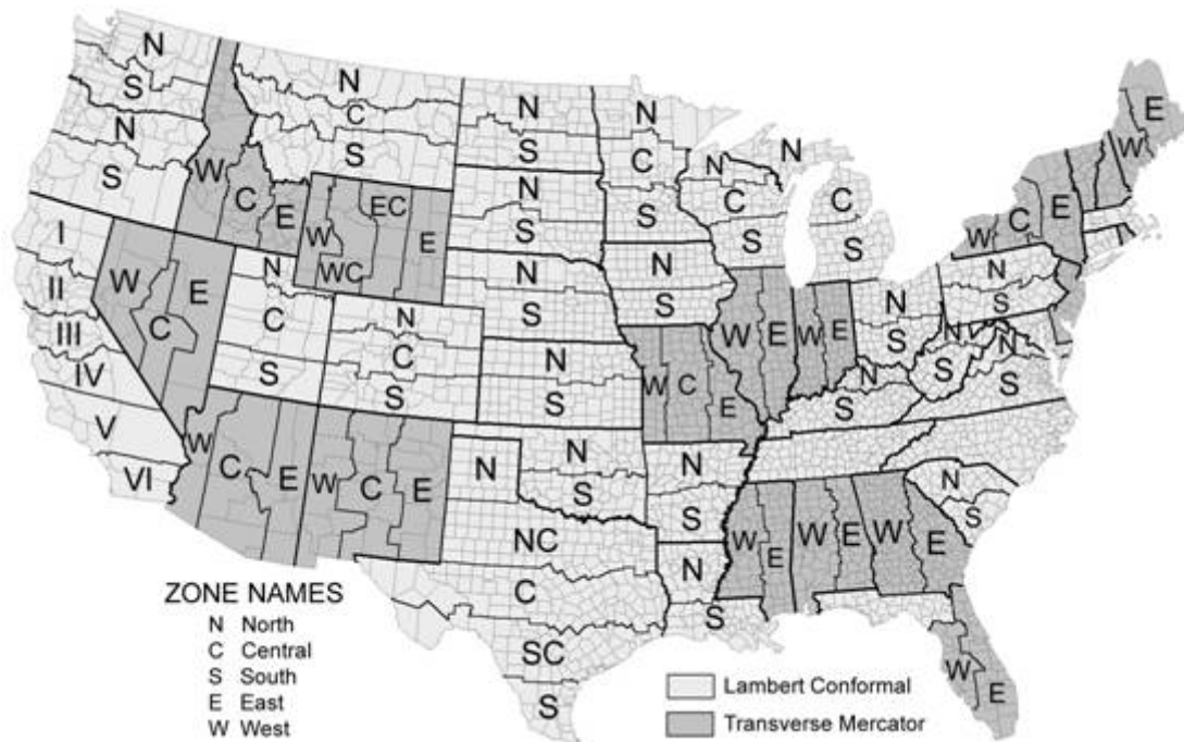
Figure 2.8. Visual depiction of the State Plane project system as displayed over the United States. http://gis.depaul.edu/shwang/teaching/geog258/Grid_files/image002.jpg
