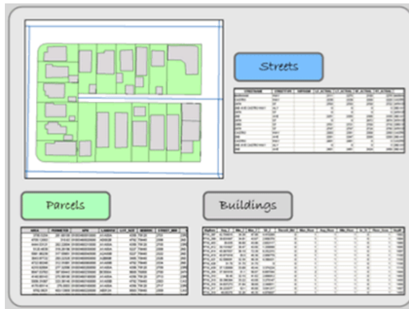
Figure 1.6. Each feature in the layers above has a spatial location and attribute data, which describes the individual feature. GIS Commons. http://giscommons.org/introduction-concepts/
