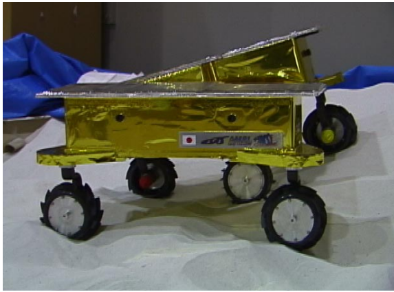
(a) The Micro5 rover prototype with PEGASUS system in a mobility test on silica sand
