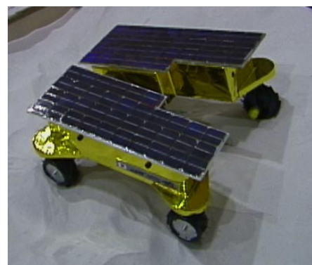
Fig.1 Micro5: prototype micro planetary rover
