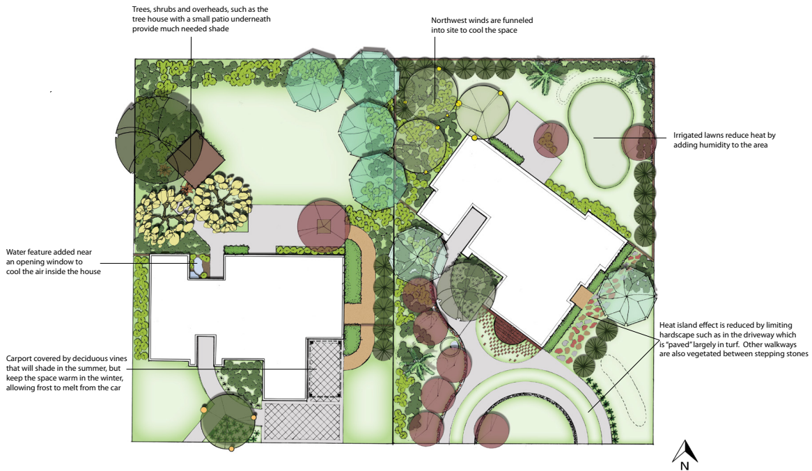
FIGURE 8. Passive design techniques applied in Bakersfield. Design by Trevor Cassidy.
