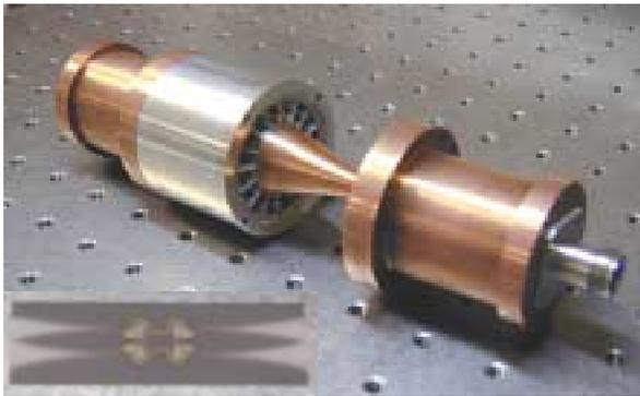
Fig. 6. Open view of the passive coaxial waveguide combiner.
