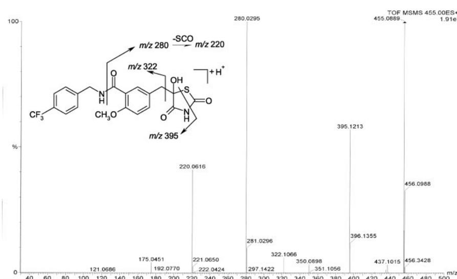
Fig. 7. MS/MS spectrum of metabolite **M24** obtained on a Q-ToF instrument and the assignments of the fragment ions. The accurate mass measurement data are summarized in Table 2.
