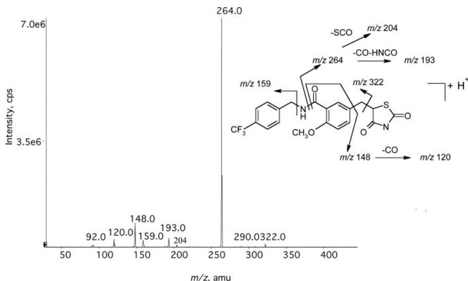
Fig. 5. MS/MS spectrum of MK-0767 and tentative assignments of the fragment ions.
