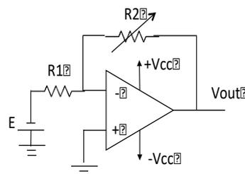
Figure 2: Reading electronics for the resistive flex sensor's (R2) outputs. The RFS behaves in feedback of an OpAmp.
