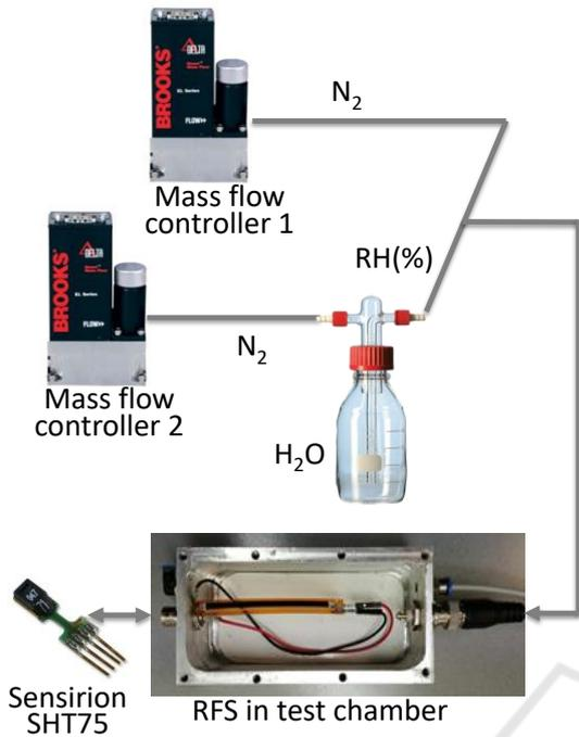
Figure 4: Set-up to investigate the different sensitivity of the RFS for three different bending conditions of the bubbling water.
