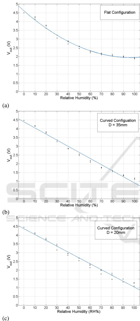
Figure 6:  $V_{out}$  vs. RH% for RFS in (a) flat, (b) 35mm diameter-support ( $R^2=0.9852$ ), (c) 20mm diameter-support bending condition ( $R^2=0.9855$ ).
