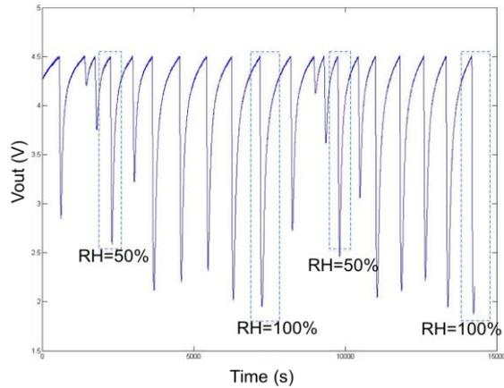
Figure 5: Sequence of dynamic responses in the time (seconds) domain, registered for the output voltage of the sensor system (flex resistance in flat configuration + electronic interface) when different RH% values are flown into the sensor cell.
