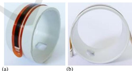
Figure 3: (a) Lateral and (b) side view of the RFS placed on a 20mm diameter support.
