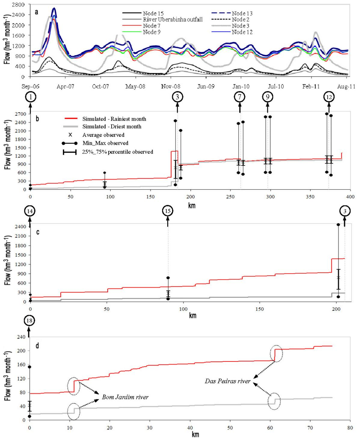
**Figure 5.** a) Variation of the simulated flow over the period of calibration and validation at the main points in the basin. Longitudinal profile of the simulated flows in the driest and rainiest months, with values of average, maximum and minimum flow rates observed and 25-75% percentiles observed in b) Araguari River, c) Quebra-Anzol River, and d) Uberabinha River.
