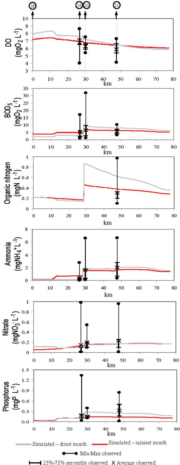
**Figure 7.** Longitudinal profile of the simulated quality parameters for the rainiest and driest months, and values of average, maximum and minimum flow rates observed and 25-75% percentiles observed in the period of calibration and validation in Uberabinha River.
