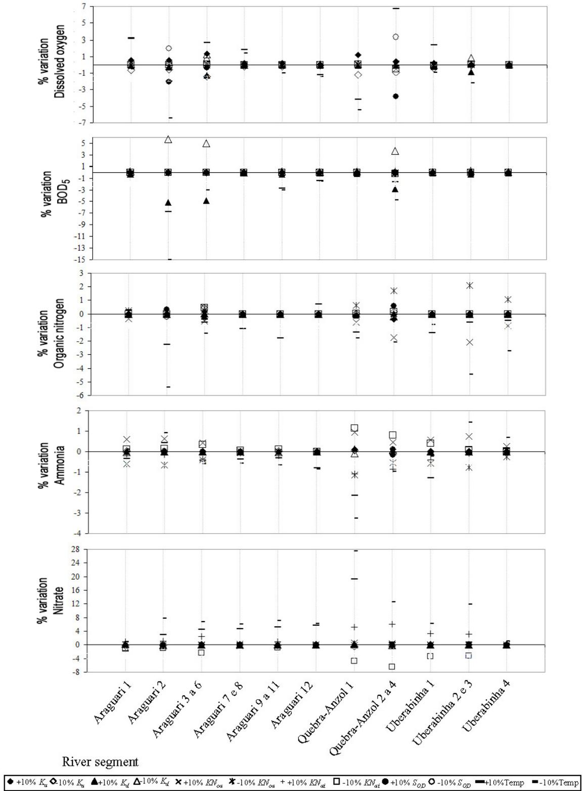
**Figure 10.** Sensitivity Analysis – Percentages of variation of the DO, BOD<sub>5</sub>, organic nitrogen, ammonia and nitrate parameters as a function of the segments of river.
