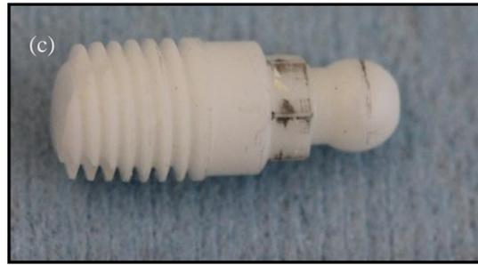
**Figure 2.** Clinical examples of fractured zirconia implants: (a,b) implants fractured during surgery; (c) implants fractured after prosthodontic loading.
