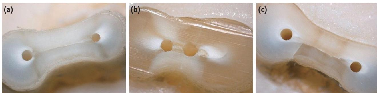
**Figure 1.** Representative stereomicroscopic images of the root cross-sections. (a) 'no crack'; (b) and (c) 'crack' formation.
