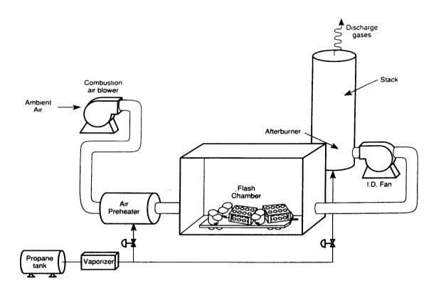
Figure 1 Hot Gas Decontamination Process Schematic
