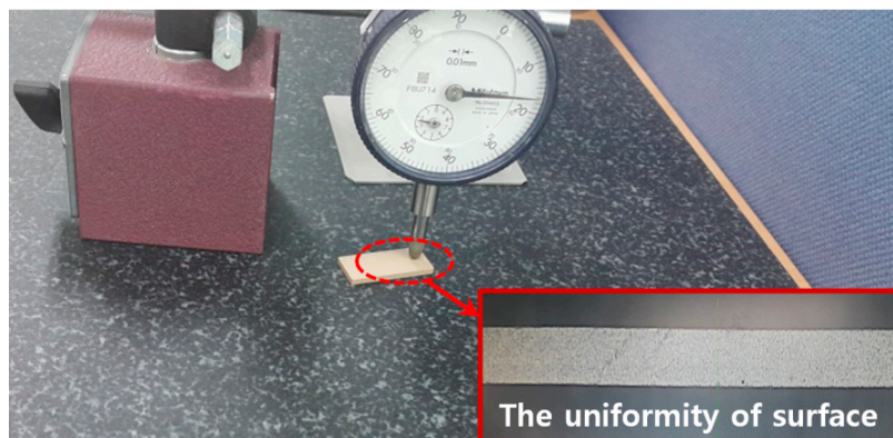
Figure 3. Measuring PTC element thickness.
