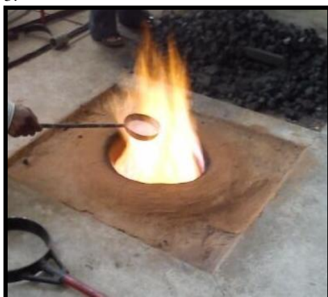
Figure 3: Adding flux to molten metal
