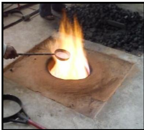
Figure 3: Adding flux to molten metal
