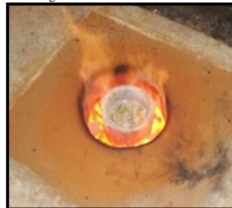
Figure 2: Coke fired pit furnace
