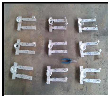
Figure 5: Test castings after fettling
