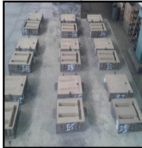
Figure 1: Dry sand molds prepared for pouring
