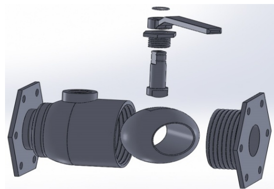
Figure-6. DFMA of flow control valve side entry design with 7 components.
