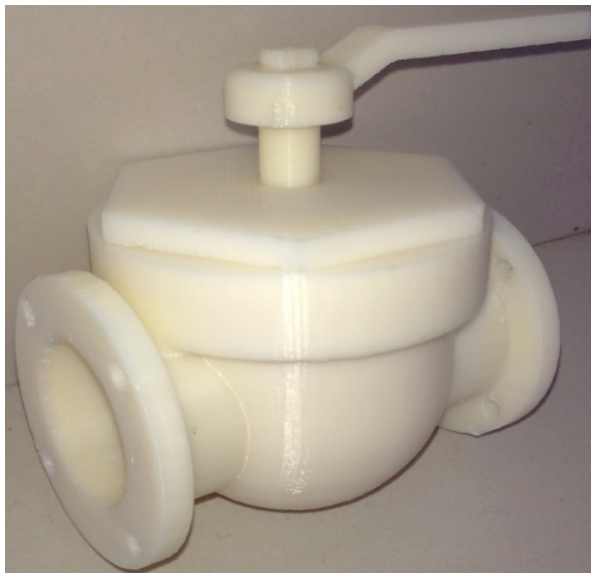
Figure-9. DFMA of the flow control valve top entry design manufactured by rapid prototyping.
