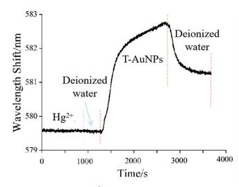
**Figure 5.** Sensing of  $Hg^{2+}$  ions with the fiber-optic SPR sensor: real time sensing process of  $Hg^{2+}$  ions.
