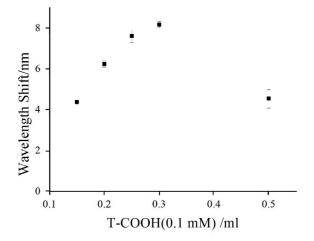
Figure 8. The optimization volumes of T-COOH (0.1 mM) for its modification on Au NPs.
