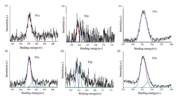
**Figure 3.** The XPS spectra of Au NPs/AET and Au NPs/T: (a) N1s spectrum of the Au NPs/AET; (b) S2p spectrum of Au NPs/AET; (c) O1s spectrum of the Au NPs/AET; (d) N1s spectrum of the Au NPs/T; (e) S2p spectrum of Au NPs/T; (f) O1s spectrum of the Au NPs/T.
