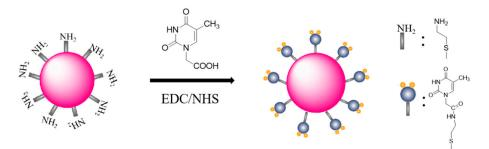
**Figure 2.** A schematic illustration of the fabrication of the thymine-modified gold nanoparticles (Au NPs/T).
