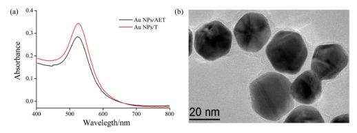
**Figure 4.** The characterization of Au NPs: (**a**) UV–vis absorption of Au NPs/AET and Au NPs/T; (**b**) TEM image of Au NPs/T.
