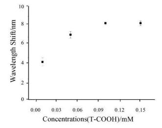
**Figure 7.** The optimization concentrations of T-COOH for the modification of a fiber-optic sensing surface.
