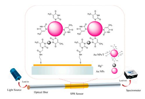
**Figure 1.** A schematic of the thymidine-functionalized fiber-optic surface plasmon resonance (SPR) biosensor for Hg<sup>2+</sup> detection.
