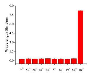
Figure 10. SPR responses for different metal ions based on sandwich structure.
