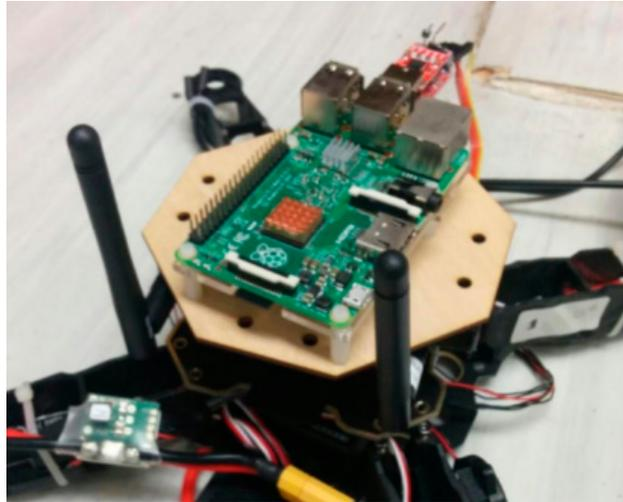
**Figure 8.** Onboard computer module.
