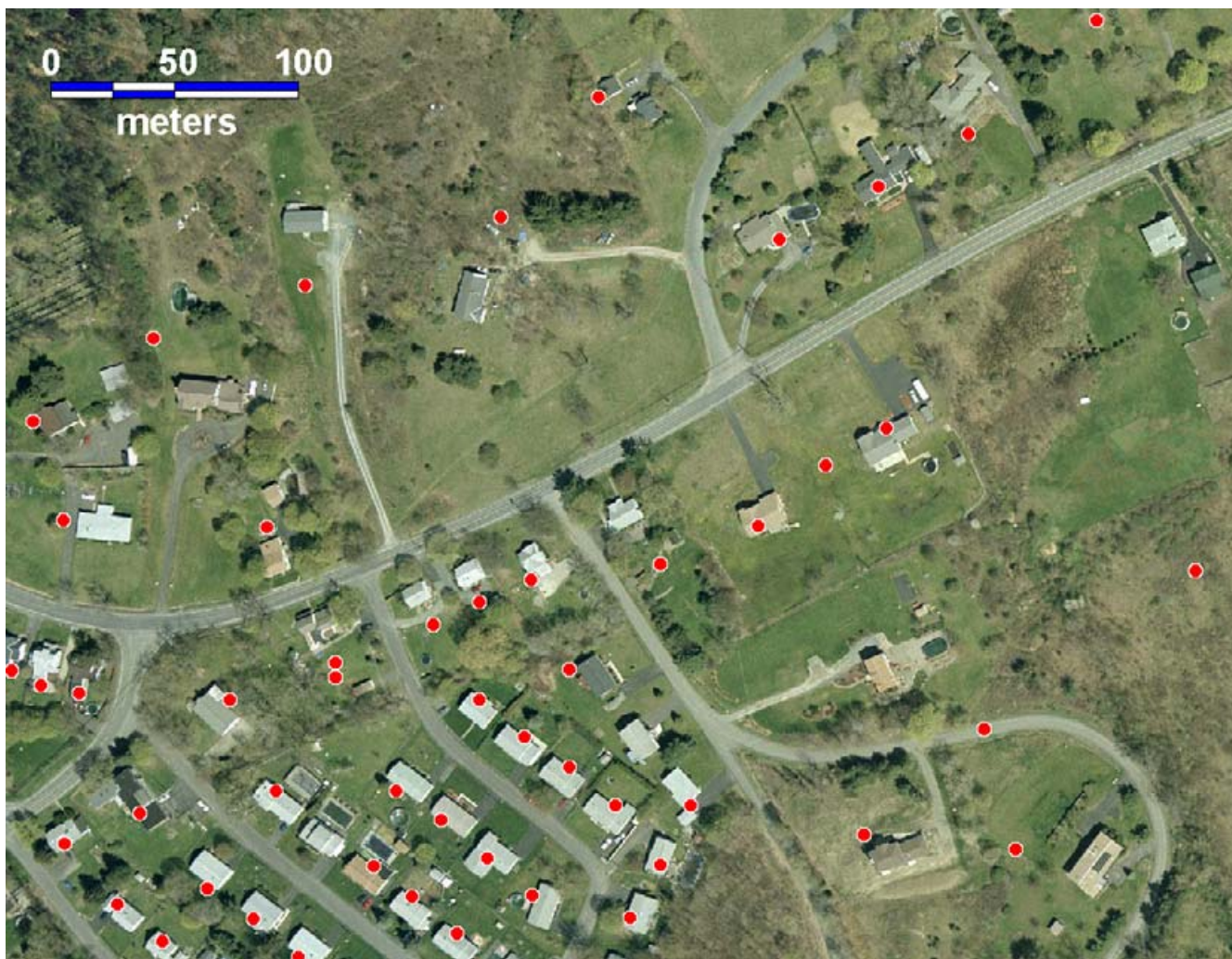
Figure 1 Residential parcel points and high resolution aerial imagery. Property parcel points from the NYSORPS. Each circle represents the approximate centroid of a property parcel classified as residential.
