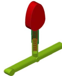
Fig. 18: Cam unit and spring follower
