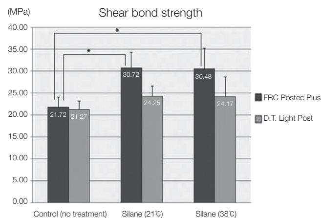
**Fig. 3.** Shear bond strength of the FRC Postec Plus and the D.T. Light Post as a function of the surface treatment.
