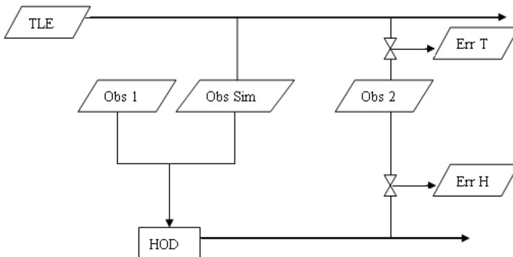
**Figure 1.** Flow Chart for the orbit determination and assessment process --- TLE and HOD stand for space debris orbits, while Obs-1 and Obs-2 represent observation data in separated passes.
