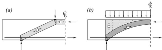
Fig. 2—Stress fields according to theory of plasticity for one-way slabs in case of: (a) concentrated loads; and (b) distributed loads.
