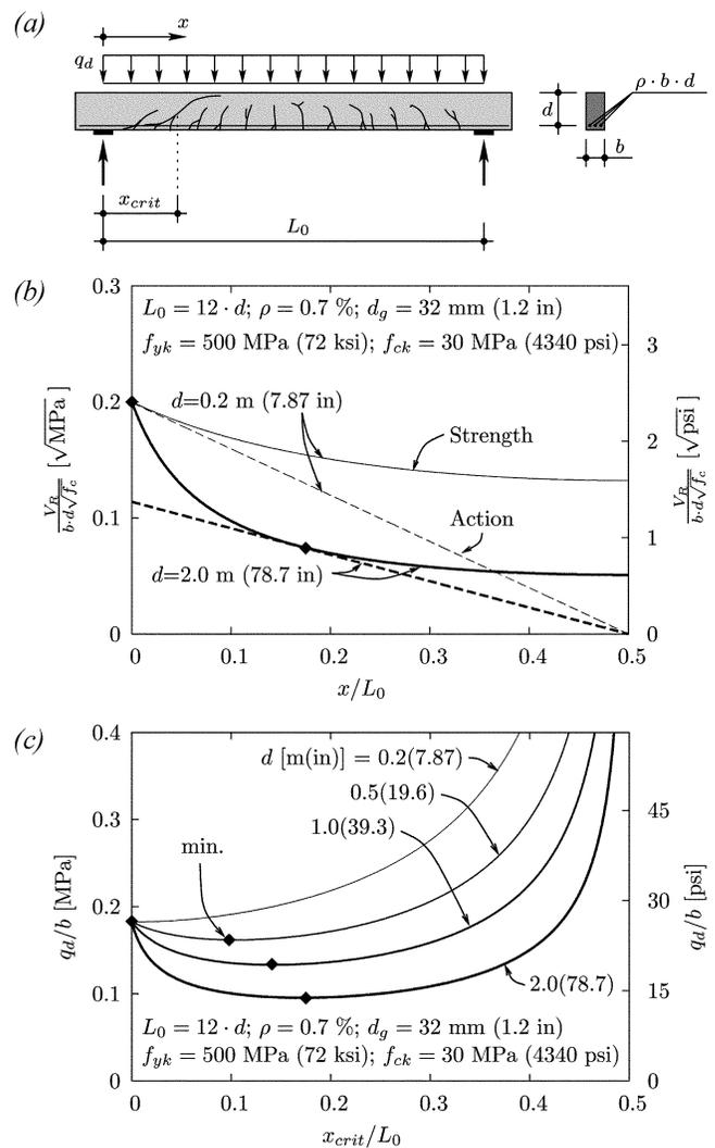
Fig. 12—Shear critical section for distributed loading: (a) geometry and mechanical parameters investigated; (b) location of critical sections (tangent between strength and action lines) for two effective depths; and (c) required load to develop shear failure at each section of beam and minimum (indicating shear critical section) for various effective depths.
