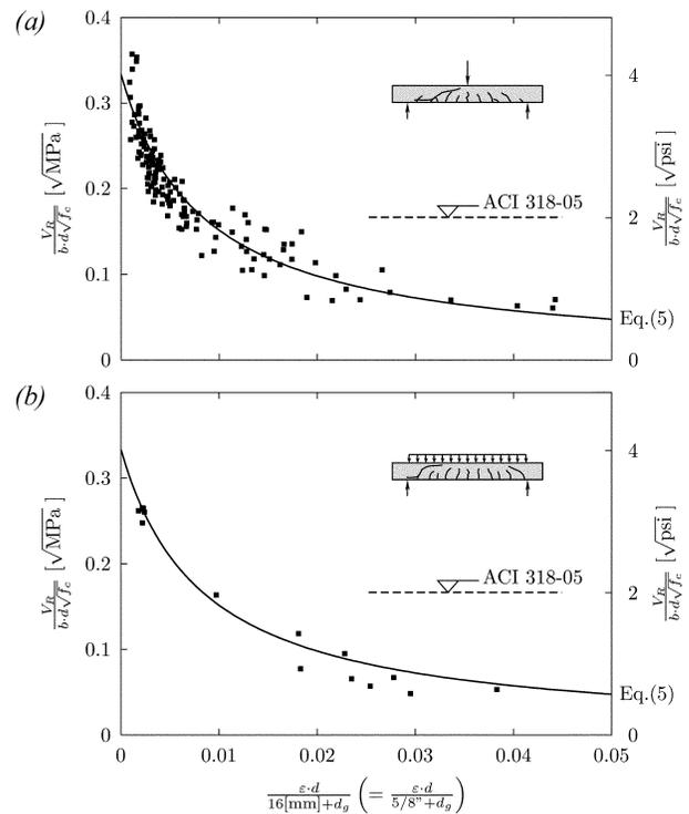
Fig. 10—Comparison of Eq. (5) and ACI 318-05<sup>24</sup> with test results for normal and high-strength concrete members: (a) concentrated loading; and (b) distributed loading.
