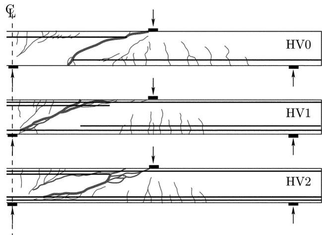
**Fig. 11—Cracking pattern in Beams HV0, HV1, and HV2<sup>37</sup> with reinforcement cutoffs.**
