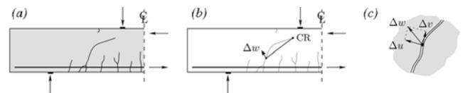
Fig. 7—Aggregate interlock after development of critical shear crack: (a) actual crack pattern; (b) center of rotation (CR) assuming two rigid bodies; and (c) normal ( $\Delta u$ ) and tangential ( $\Delta v$ ) relative displacements between lips of crack.
