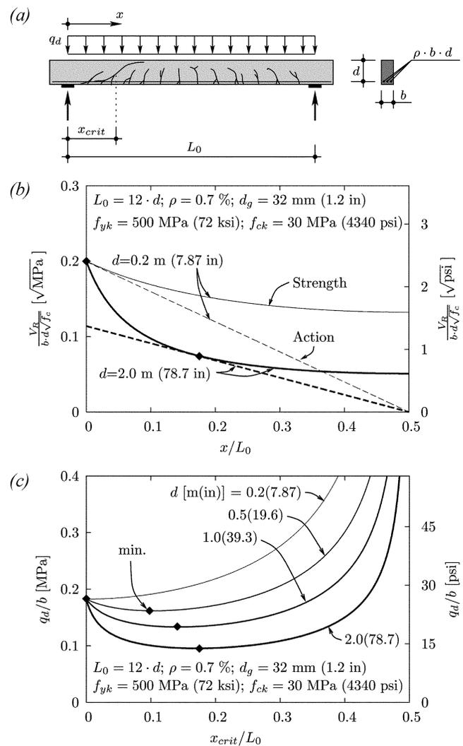
Fig. 12—Shear critical section for distributed loading: (a) geometry and mechanical parameters investigated; (b) location of critical sections (tangent between strength and action lines) for two effective depths; and (c) required load to develop shear failure at each section of beam and minimum (indicating shear critical section) for various effective depths.
