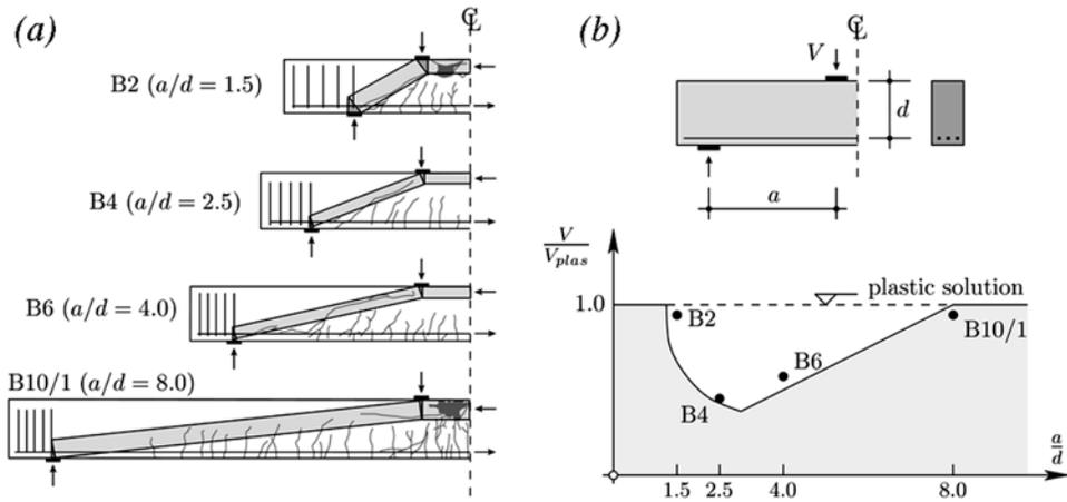
Fig. 4—Influence of  $a/d$  on shear strength: (a) Tests B2, B4, B6, and BP10/1 by Leonhardt and Walther,<sup>16</sup> cracking pattern and theoretical strut position; and (b) Kani's valley, comparing actual strength with failure load according to theory of plasticity.
