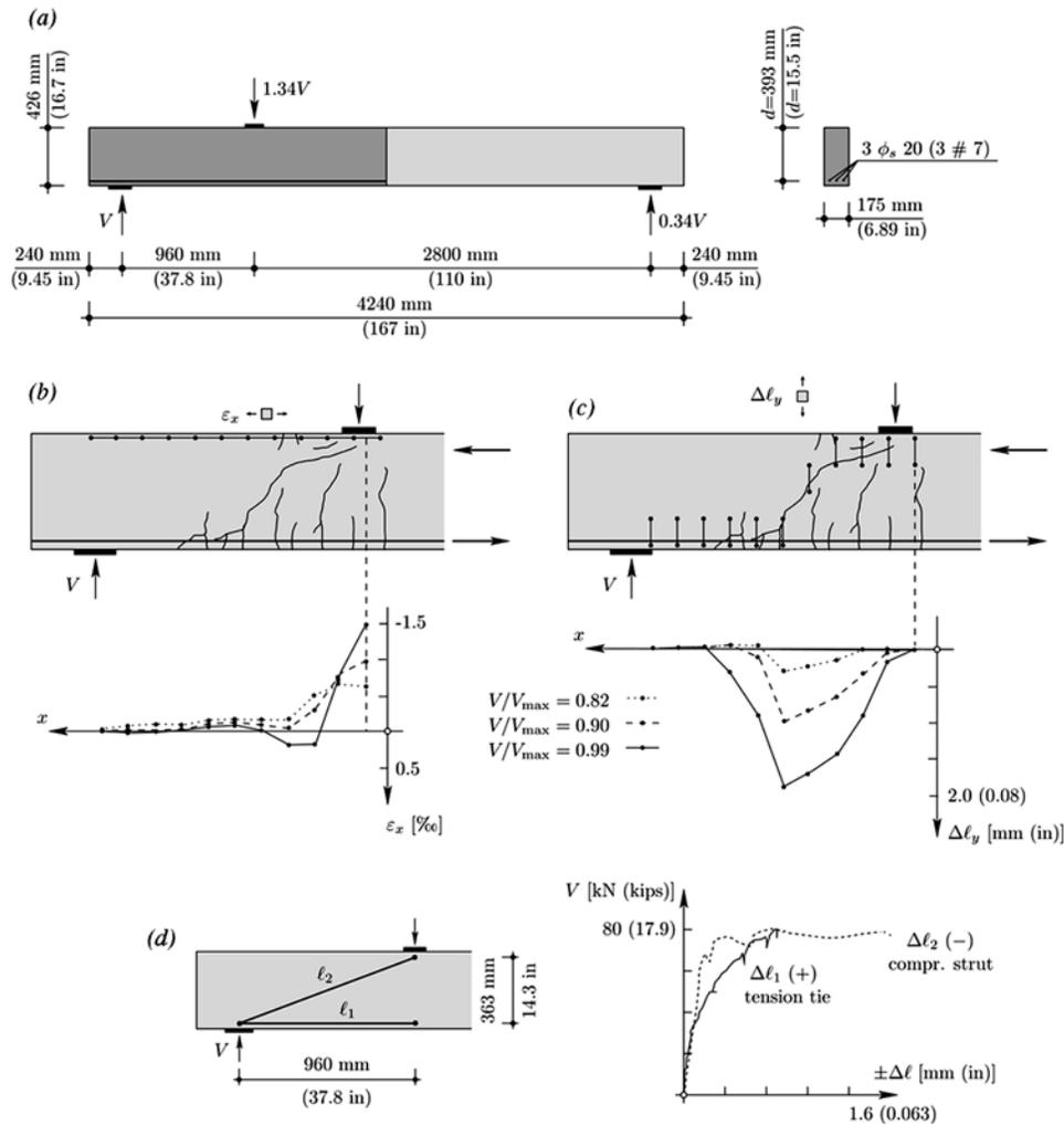
Fig. 8—Test BP0 by Muttoni and Thürlimann<sup>17</sup> ( $f_c = 30.5 \text{ MPa}$  [4.42 ksi];  $d_g = 16 \text{ mm}$  [5/8 in.]): (a) test setup; (b) crack pattern and horizontal strains along top fiber (points of measurement indicated); (c) crack pattern and vertical elongation along diagonal crack (points of measurement indicated); and (d) measured elongations in directions of compression strut and of tension tie.
