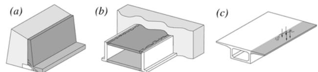
*Fig. 1—Some structural elements without shear reinforcement working predominantly as one-way slabs (only shear cracks drawn): (a) wall and foundation of retaining wall; (b) upper and lower slabs of cut-and-cover tunnel; and (c) deck slab of bridge.*
