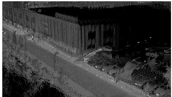
Figure 1: 3D point cloud visualization of a section of Begbroke Science Park before and after calibration. The 2D LIDAR is angled downwards by 8^\circ , and therefore covers a volume up to 2m above the ground plane. In the lower image, good calibration is evident between the two point clouds, particularly on sections of the building, lamp posts and automobiles.
