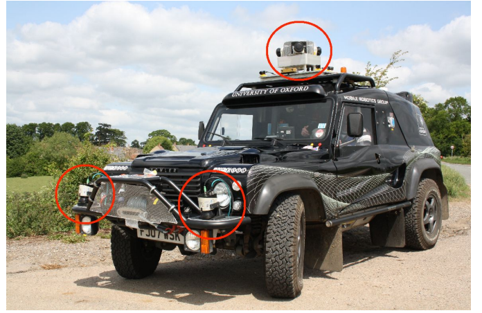
Figure 2: The Wildcat vehicle has a spinning 3D LIDAR on the roof, and two 2D LIDARs on the front bumper at different elevation angles (sensors circled in red). The INS system is mounted over the rear axle.
