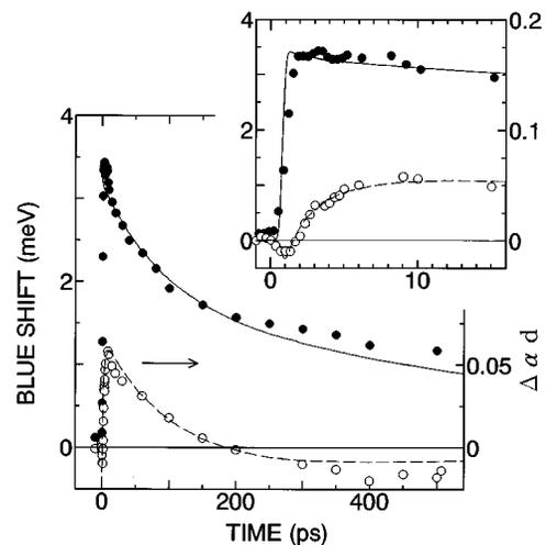
FIG. 6. Temporal changes of the blue energy shift of the  $Z_3$ -exciton band ( $\bullet$ ) and the optical gain ( $\circ$ ). The inset shows the temporal changes on the expanded time scale. The solid and dashed lines show  $N_{ex} + 2N_m$  and  $N_m - kN_{ex}$  obtained from the result of the simulation with  $\lambda = 1.5$ , respectively.
