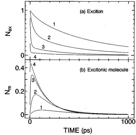
FIG. 1. Numerical solutions of rate equations shown in the text under the initial conditions,  $N_{\text{ex}}(t=0)=1$  and  $N_m(t=0)=0$ . Curves 1, 2, 3, and 4 correspond to  $\alpha=1, 10, 100$ , and  $1000/\text{ns}$ , respectively. The upper figure shows the temporal change of the exciton density, while the lower figure that of the excitonic molecule density. The other parameters used are  $\tau_{\text{ex}}=800 \text{ ps}$  and  $\tau_m=70 \text{ ps}$ .
