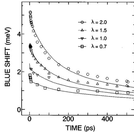
FIG. 7. Temporal change of the blueshift of the  $Z_3$ -exciton band for four excitation densities, 1.6  $\text{mJ}/\text{cm}^2$  ( $\circ$ ), 810  $\mu\text{J}/\text{cm}^2$  ( $\Delta$ ), 320  $\mu\text{J}/\text{cm}^2$  ( $\nabla$ ), and 160  $\mu\text{J}/\text{cm}^2$  ( $\square$ ). Solid lines indicate  $N_{\text{ex}}+2N_m$  obtained from the results of the simulation with  $\lambda=2.0$ , 1.5, 1.0, and 0.7, respectively.
