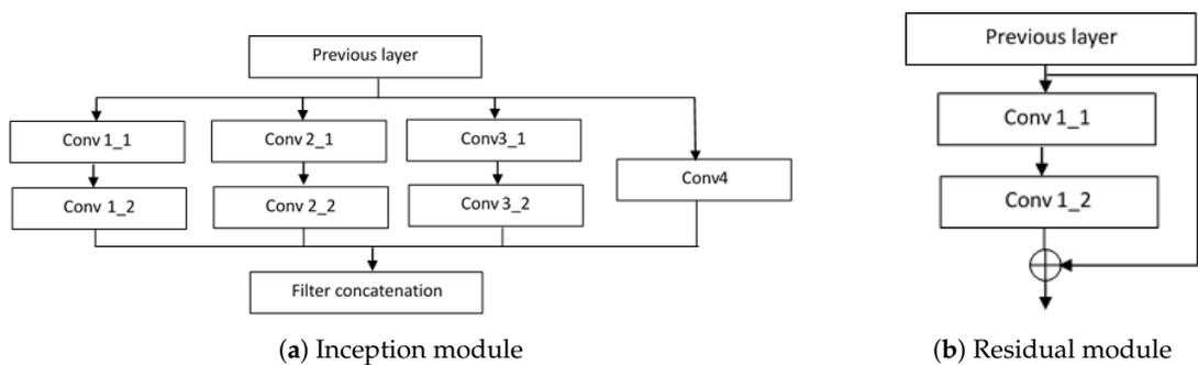
**Figure 4.** Composition modules in the proposed HSN architecture. (a) Inception module; (b) Residual module.
