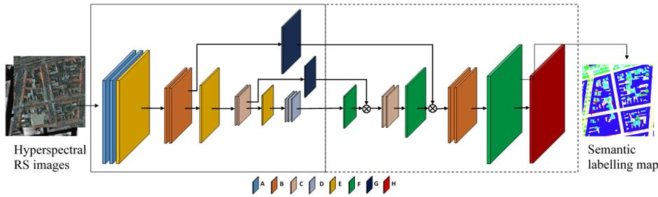
**Figure 3.** The proposed hourglass-shaped network (HSN) architecture. A and B are convolutional layers; C and D are inception modules; E is the max pooling layer; F is the transposed convolutional layer; G is the residuals modules; H is the loss layer.
