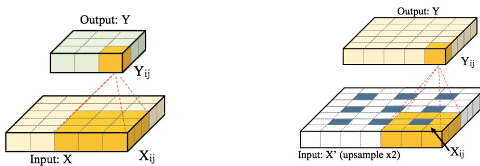
(a) Convolutional layer: the input size is  $W_1 = H_1 = 5$ ; the receptive field  $F = 3$ ; the convolution is performed with stride  $S = 1$  and no padding ( $P = 0$ ). The output  $Y$  is of size  $W_2 = H_2 = 3$ .
