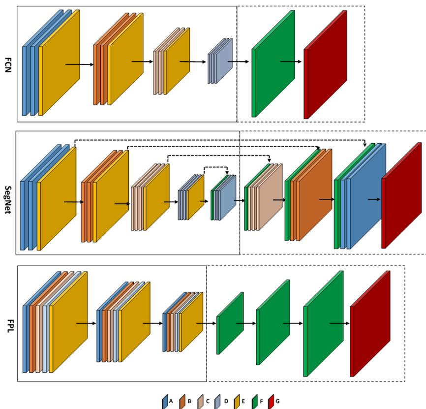
**Figure 2.** The fully-convolutional network (FCN) [21], SegNet [19] and full patch labeling (FPL) [22] network designs. A, B, C and D are convolutional layers; E is a pooling layer; F is a transposed convolutional layer or unpooling layer (in SegNet); G is a loss layer.
