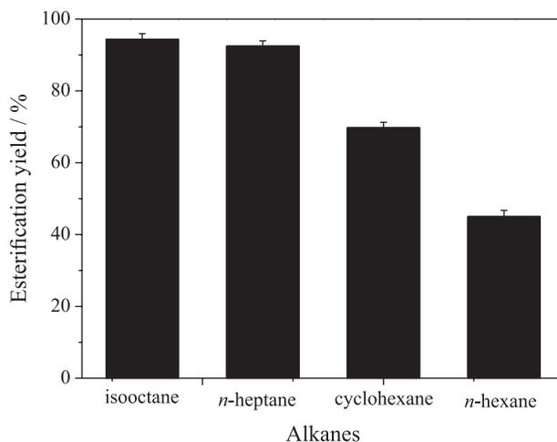
**Figure 5.** Effect of different kinds of microemulsion system on esterification (reaction conditions: molar ratio (alcohol/acid) 4,  $w_0$  3.3, time 4 h, lipase 120 mg  $g^{-1}$ ).
