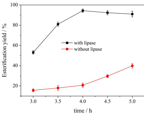
**Figure 3.** Effect of reaction time on esterification catalyzed by CRL and without CRL in DBSA microemulsion system (reaction conditions: molar ratio (alcohol/acid) 4,  $w_0$  3.3, lipase 120 mg  $g^{-1}$ ).
