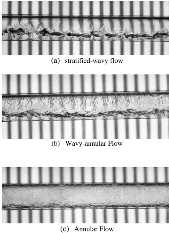
Fig. 4 Flow patterns in horizontal microfin and plain tube
