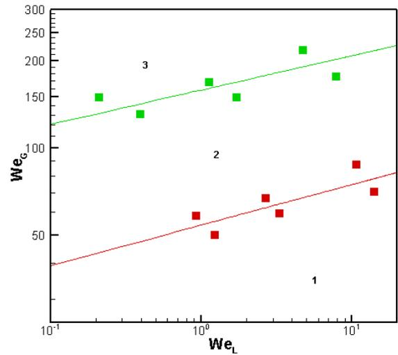
1-Churn Flow; 2-Wavy Annular Flow; 3-Annular Flow
