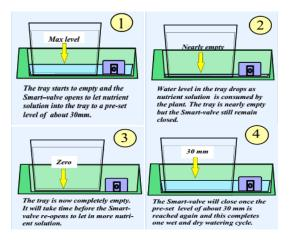
Figure 2. Water circulation of Autopot System(Fah, 1996)
