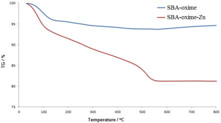
Fig. 2: Thermal gravimetric analysis (TGA) of (a) SBA-oxime and (b) SBA-oxime-Zn.
