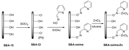
Scheme 1: Synthesis of zinc-anchored SBA-15
