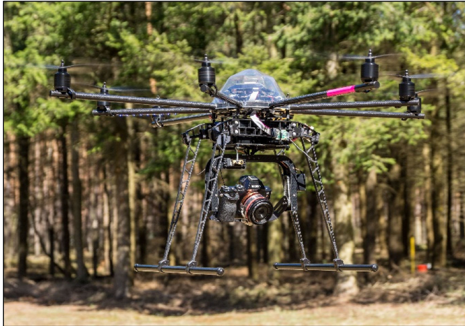
Figure 4. OctoXL 6S12 Octocopter mounted with a fixed lens Sony A7r RGB camera.
