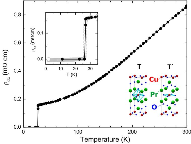
**Figure 1.** (Color online) Main panel: Temperature dependence of the in-plane dc resistivity  $\rho_{dc}$  of the  $T'$ -PCO film. In the right-hand corner schematic diagrams illustrate the  $T$  and  $T'$  structures. Inset: A close-up of the dc resistivity around the superconducting transition. The dc measurements were performed twice: on the fresh film [solid (black) symbols] and after completion of all optical measurements [open (grey) symbols].
