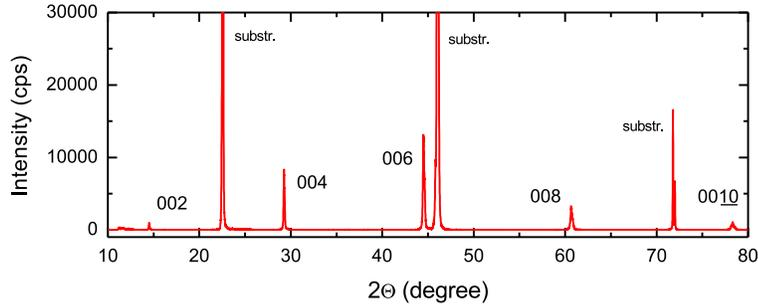
**Figure 2.** (Color online) X-ray diffraction pattern of a  $c$ -axes oriented PCO film on  $\text{DyScO}_3$  substrate. Diffraction peaks coming from the substrate are marked as “substr.” The lattice constant along the  $c$ -axes calculated from the positions of the film peaks is 12.20 Å, indicating the optimal oxygen reduction and the proper  $T'$  structure [4].
