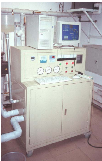
Fig. 7: Different thermal response test rigs, from above: Early rig from Landtechnik Weihenstephan, rig built by UBeG for export to China, light rig built by hp system tech in South Korea, laboratory rig at Beijing University of Technology, China
