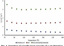
Fig. 4. Variation of specific heat capacity ( $C_p$ ) of citriodora oil, N-(2-aminoethyl)-oleamide and gel as a function of temperature
