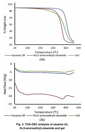
The closer scrutiny of the Fig. 3a and 3b, TGA-DSC of sesame oil, N-(2-aminoethyl)oleamide and gel reveals quite a similar pattern of decomposition as well as heat flow as a function of temperature with the previous mustard oil systems.
