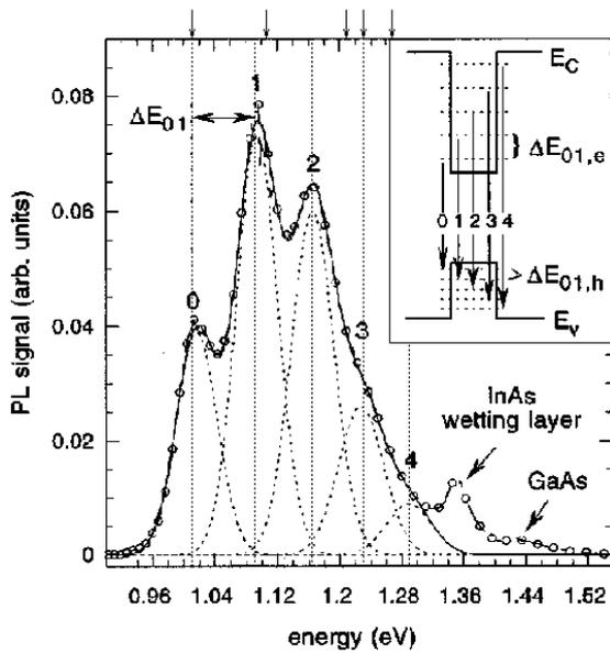
**Fig. 1** Comparison between our predicted transition energies (top arrows) and the experimental PL spectrum by Schmidt et al. [5] [“Copyright (1996) by the American Physical Society”].
