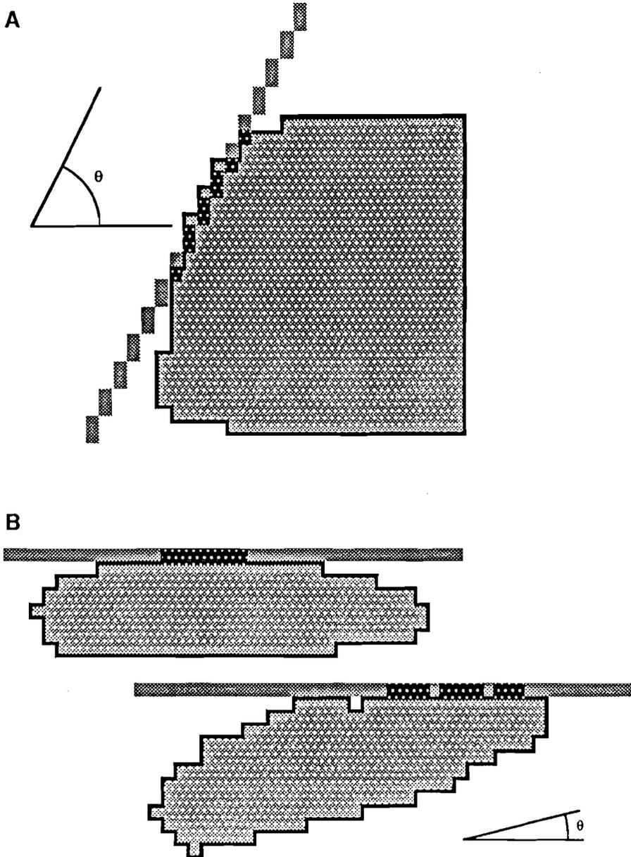
**FIG. 7. A:** Digitization of an image along with rotation of test lines may result in errors in intercept counts. In this case, there are six intercepts where there should be only two. **B:** Rotation of a digitized image within computer memory, keeping test lines fixed, can also introduce multiple intercept counts. As with (A), this rotation results in six intercepts where there should be only two.
