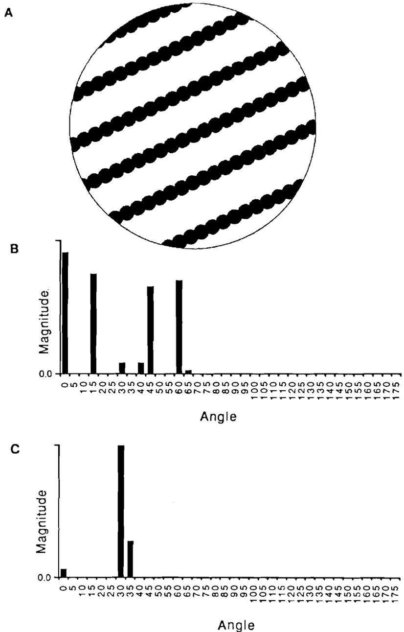
**FIG. 8. A:** Sample pattern with one structural direction of orientation and microstructural features. **B:** Corresponding normalized phase distribution with test line width = 2 pixels. **C:** Normalized phase distribution with test line width = 5 pixels. Units are intercepts per unit length.
