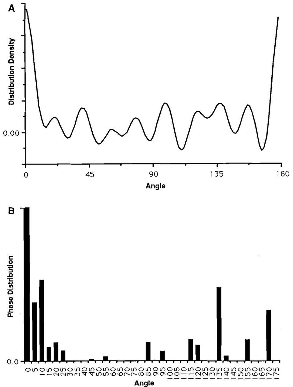
**FIG. 4. A:** Normalized distribution density plot for sample pattern of Fig. 1. **B:** Normalized phase distribution plot. Both plots are generated using maximum degrees of freedom in the respective procedures. Units are intercepts per unit length.
