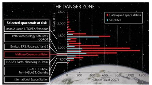
**Figure 2 | Levels of space debris as of 2007.** Orbits with more space debris have higher risks of impact. Space debris in higher orbits requires the most time to fall back to Earth. Reproduced with permission from G. Forden, Massachusetts Institute of Technology.
