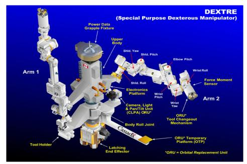
**Figure 1 | Dextre, the Canadian Space Agency newest automation.** Equipped with tools and cameras, Dextre will be busy conducting maintenance work on the International Space Station's interior. Reproduced with permission from the Canadian Space Agency.
