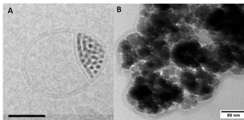
**Figure 7.** Cryo-TEM (transmission electron microscopy) micrographs of (A) lipid bilayer splitting around incorporated MNPs (scale bar = 50 nm). Reprinted from [151] with permission of ACS Publications. (B) Protein corona of bovine serum albumin formed at the surface of MNPs (unpublished own data).
