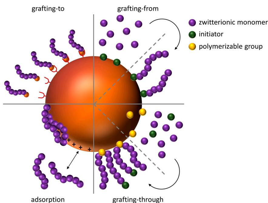
**Figure 3.** Schematic representation of different grafting methods of polymers to nanoparticle surfaces.
