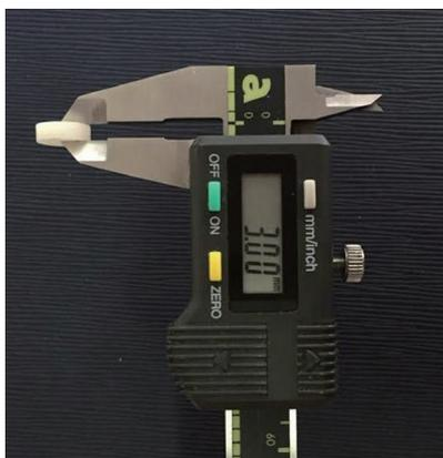
Fig. 2. Measurement of test specimens.
