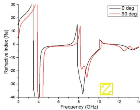
**Figure 6.** Real magnitude of the refractive index ( $\eta$ ) vs. the frequency of the 0-degree and 90-degree rotated unit cell.
