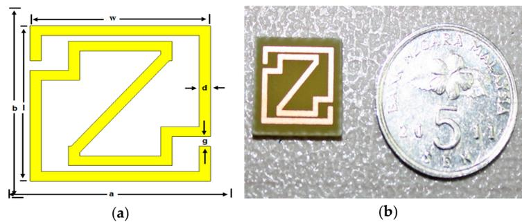
**Figure 1.** Metamaterial unit cell: (a) proposed geometry; (b) fabricated geometry.
