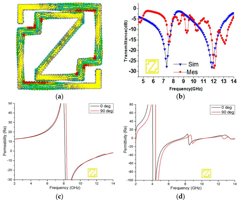
**Figure 5.** (a) Surface current density at 11.84 GHz; (b)  $S_{21}$  curve for the Z-shape unit cell; the real magnitude of (c) the effective permeability and (d) the effective permittivity of a 0-degree and 90-degree rotated unit cell.
