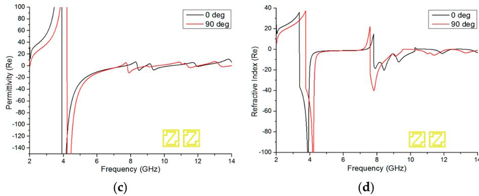
**Figure 7.** (a) 0-degree position of the  $1 \times 1$  array geometry; real magnitude of (b) the effective permeability; (c) the effective permittivity; and (d) the effective refractive index at 0-degree and 90-degree rotations of the  $1 \times 1$  array configuration.
