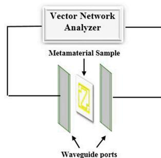
Figure 3. Experimental setup for measuring the S-parameters.
