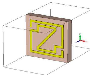
**Figure 2.** Simulation setup of the proposed Z-shape unit cell for CST Microwave Studio (CST MWS) in a free-space environment.
