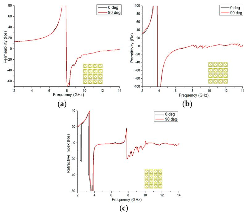
**Figure 9.** Real magnitude of (a) the effective permeability; (b) the effective permittivity; and (c) the refractive index of the 90-degree rotated  $4 \times 4$  array configuration.
