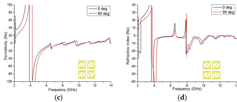
**Figure 8.** (a) 90-degree rotated  $2 \times 2$  array geometry; the real magnitude of (b) the permeability; (c) the permittivity; and (d) the refractive index of the 90-degree rotated  $2 \times 2$  array configuration.
