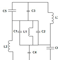
**Figure 4.** Equivalent LC circuit model of the proposed unit cell.
