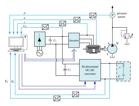
Figure 10. The system structure diagram of energy recovery and reuse.
