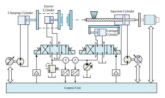
Figure 7. The hybrid control scheme of an electric-hydraulic IMM.
