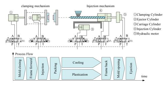
Figure 2. The composition, appearance, and process of a hydraulic injection-molding machine (IMM).
