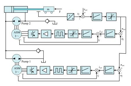
Figure 8. The principle to control differential cylinders with two speed variable pumps.
