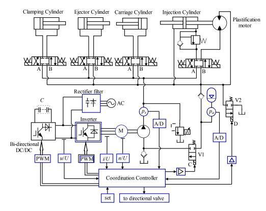
Figure 11. The principle of the coordination control strategy.
