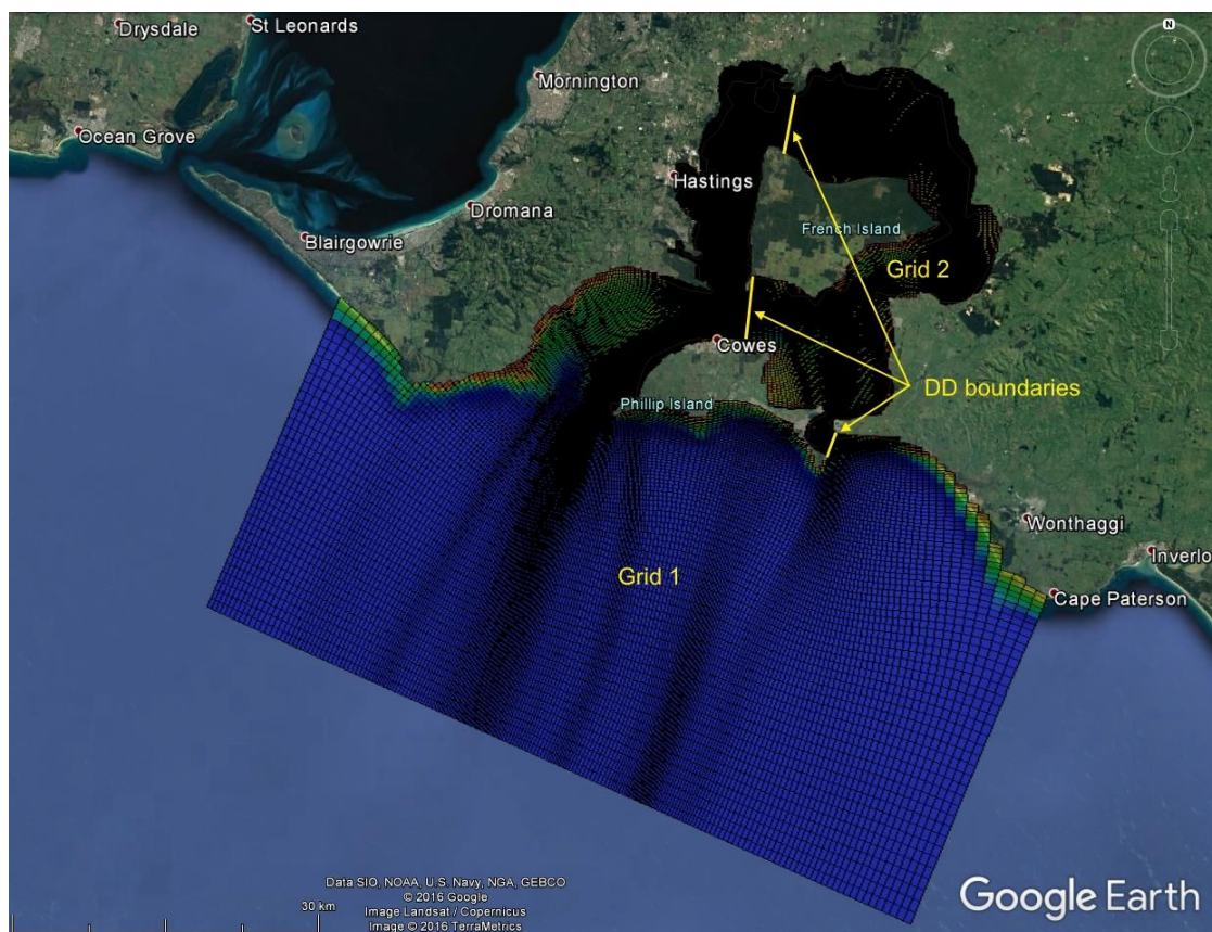
Figure 3. Extent and configuration of the Delft3D hydrodynamic model grids.
