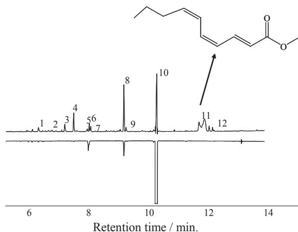
Fig. 4. Gas chromatograms of volatiles collected from live male (top) and female (bottom, inverted) *T. perditor*: 1,  $\alpha$ -pinene; 2,  $\beta$ -pinene; 3,  $\alpha$ -ocimene; 4, (E)-2-octenal; 5, (E)-2-octen-1-ol; 6, undecane; 7, nonanal; 8, dodecane; 9, (E)-2-decenal; 10, tridecane; 11, distorted peak from thermal decomposition of methyl (2E,4Z,6Z)-decatrienoate; 12, pentadecane.
