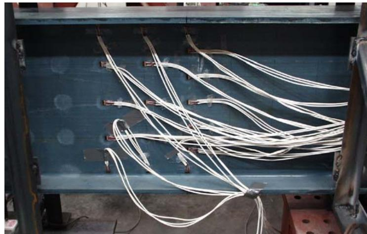
**Figure 8.** Locations of displacement sensors on the web surfaces.
