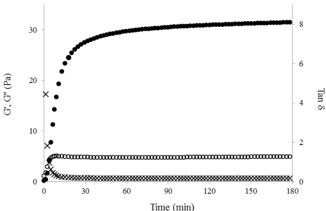
**Figure 4.** Mechanical spectrum of WEAX gel at 2% (w/v).  $G'$  ( $\circ$ ),  $G''$  ( $\bullet$ ). Measurements at 25 °C, 1 Hz and 10% strain.
