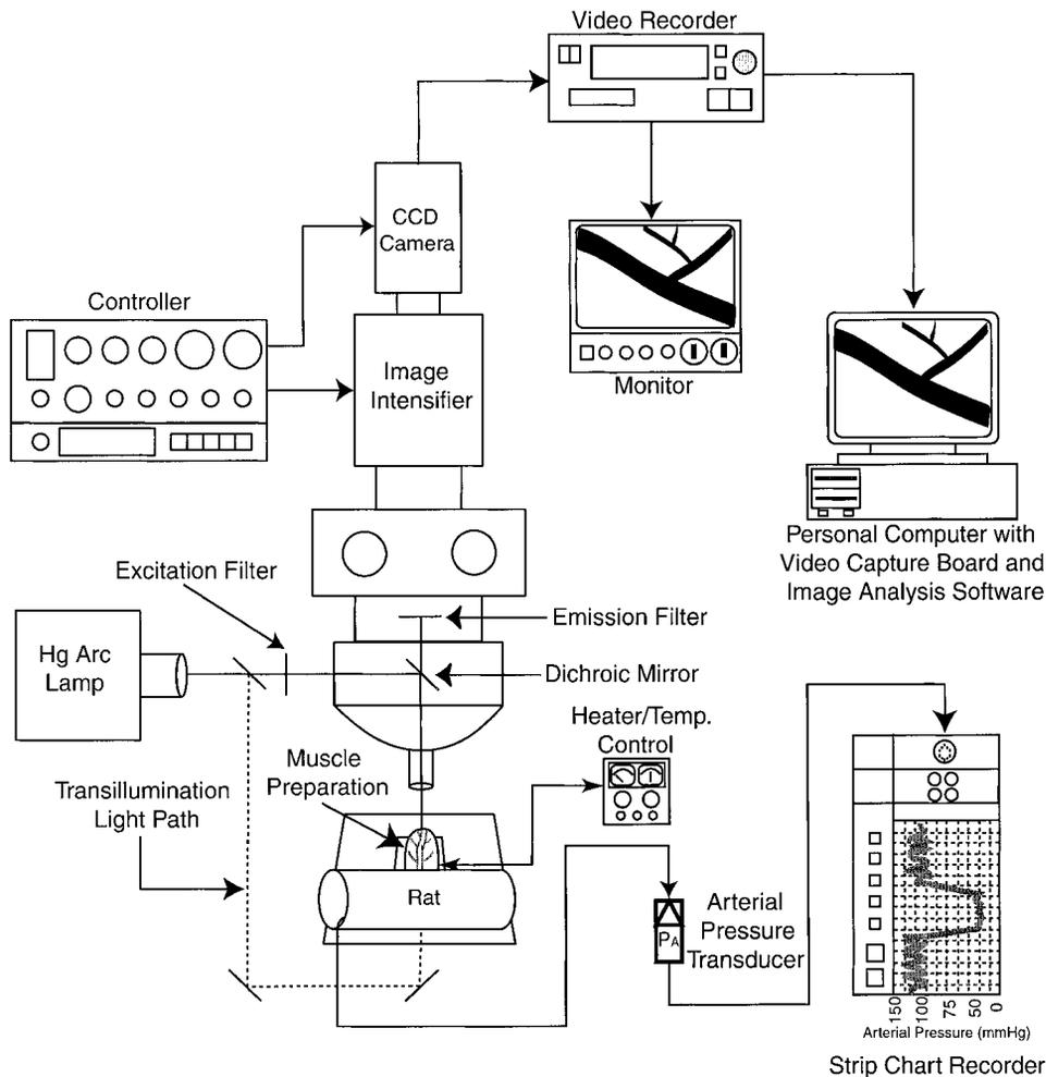
Fig. 1. Schematic diagram of the experimental setup, including an intravital microscope equipped for both trans- and epi-illumination. An externally controlled gated image intensifier allows for multiple images to be combined and recorded on a single video frame for determination of cell velocities up to 14 mm/s. A personal computer with video capture board allows the recorded image to be converted to digital format for image analysis. CCD, charge-coupled device.
