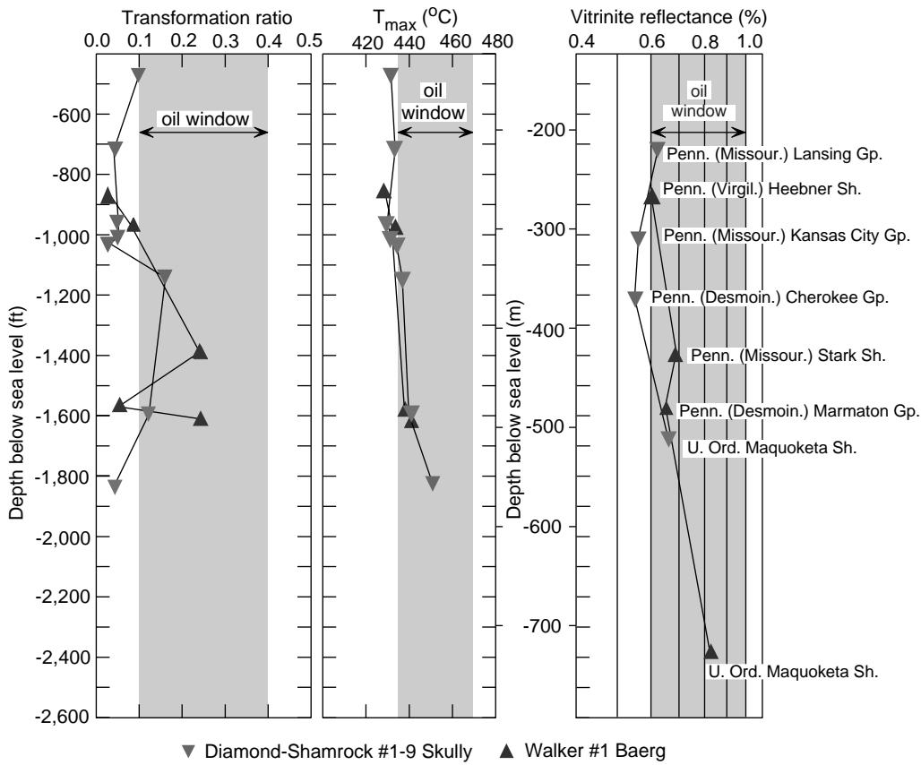
FIGURE 10. Rock-Eval and vitrinite maturation profiles for two wells near McPherson County, Kansas (refer to fig. 8 for locations).
