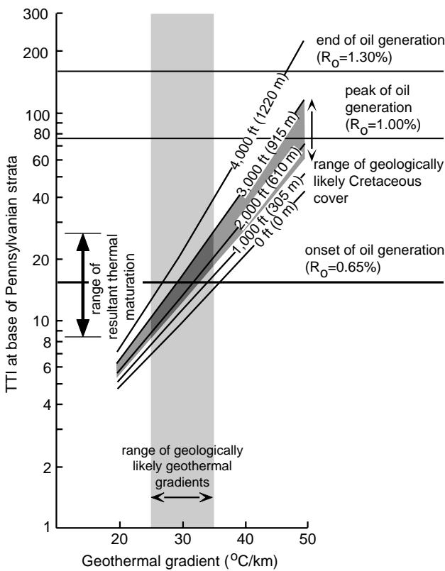
FIGURE 4. A nomogram expressing the results of TTI modeling at McPherson County as a consequence of geothermal gradient and Cretaceous burial for the base of the Pennsylvanian section. See fig. 3 for instructions for obtaining TTI. Most likely combinations of geothermal gradients and Cretaceous cover indicate the base of the Pennsylvanian section would be immature to only marginally mature with respect to oil generation.
