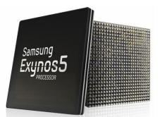
Samsung Exynos 5 Dual 2 x ARM Cortex-A15 @ 1.7GHz 2 x 32-bit DDR3-800 channels 32KB L1 + 1MB L2
