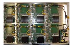
**1U Rackable blade** 8 nodes 16 GFLOPS 65 Watts 0.25 GFLOPS / W
