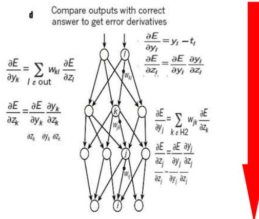
Figure 2: The implementation of backpropagation [1]
