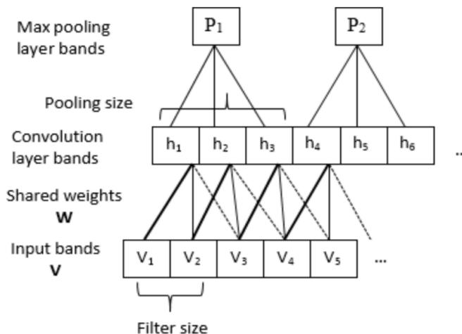
Figure 3: Convolutional neural network architecture shows one or more fully connected convolutional layers [20]
