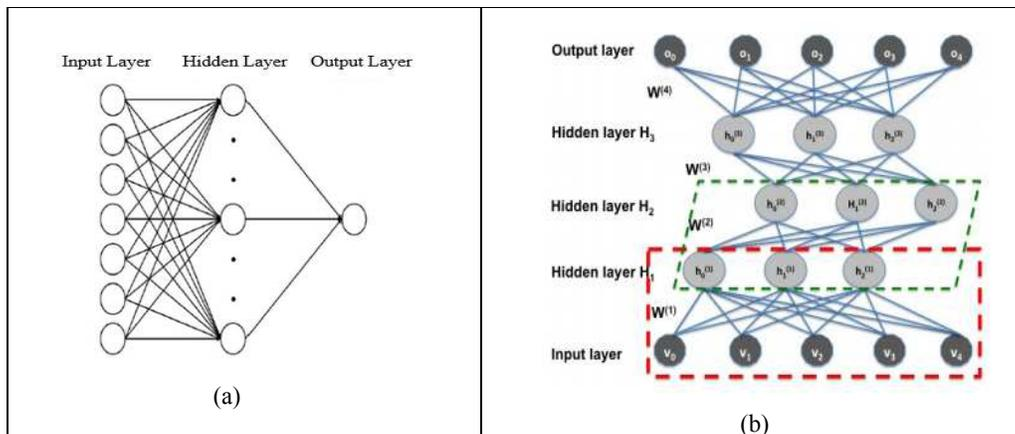
**Figure 1: The architecture between (a) conventional neural network [15] and (b) deep neural network [16]**
