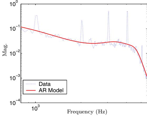
Fig. 7. Bode amplitude plot of spectral estimate of pick-up microphone signal (dotted) and AR model  $\|H_n(q)\|^2 \lambda$  (solid).
