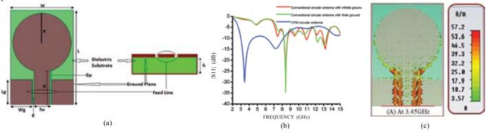
Figure 1. (a) Geometry of CPW fed circular patch antenna with its parameter, (b) Comparison of variation of |S11| with frequency of circular patch antenna in different cases, and (c) Current distribution at 3.45 GHz.
