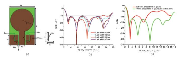
Figure 2. (a) Geometry of CPW fed circular patch antenna with L shaped slits in ground plane, (b) Comparison of variation of |S11| with frequency of circular patch antenna for different slit thickness, and (c) Comparison of variation of |S11| with frequency of patch antenna with and without L shaped slits in ground plane.
