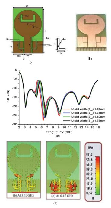
Figure 5. (a) -(b) Geometry of CPW fed circular patch antenna with U shaped slot in patch, (c) Comparison of variation of |S11| with frequency of circular patch antenna for different U slot width, and (d) Current distribution at different resonance frequencies.
