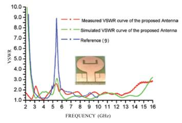
Figure 6. Comparison between VSWR curve with proposed antenna and reference antenna.
